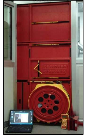
Figure 5.1 Equipments for door fan integrity test
